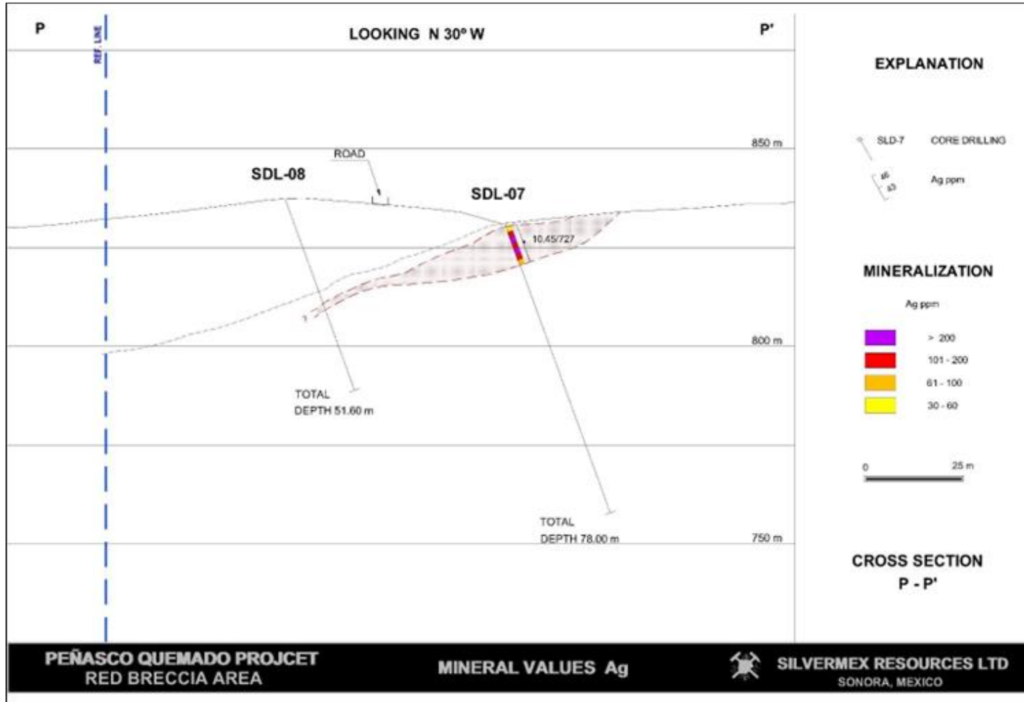
Figure 6.12 Section P to P' Drill Hole SDL-07 and SDL-08 Intersections within the San Luis/Red Breccia Area
